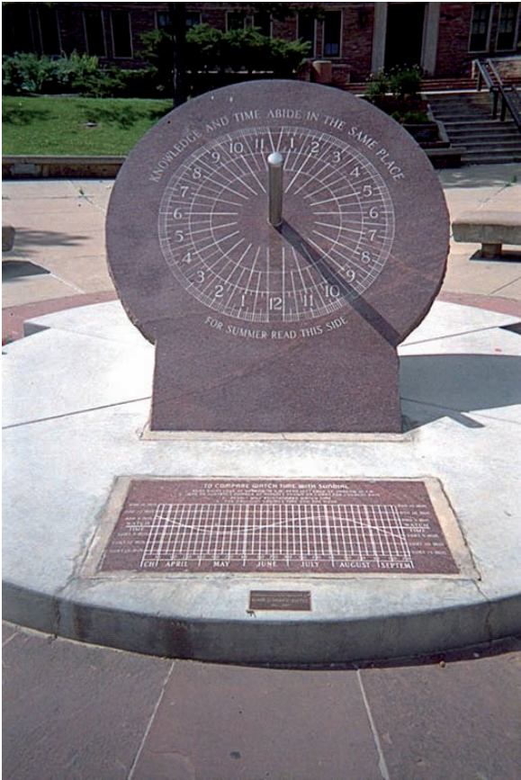
Fig. 4 Sundial at the University of Colorado. The gnomon is pointing toward the north celestial pole, which in Boulder is 30° above the horizon
